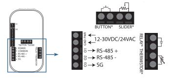
NOTE: A 120  $\Omega$  termination resistance may be added in parallel with the RS-485 +/- by moving the very top DIP switch (DIP 1) to the left position. See "DIP Configuration" section for more information.
