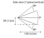
PIR can be used to automaticly wake the screen when motion is detected in the room.
